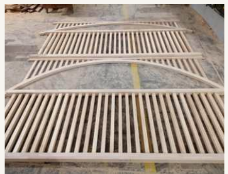
ASSEMBLED PANELS ON THE FLOOR — FR4 ARCHED WITH NO MOTIF & BS6 WITH 42 MM x 42 MM SLATS
